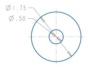
UNLESS OTHERWISE SPECIFIED, **ALB Materials Inc. DIMENSIONS ARE IN INCHES** TITLE: **TOLERANCES:** FRACTIONAL 0.030 **Ring/Tube Magnet** ANGULAR: 0.5 TWO PLACE DECIMAL 0.010 THREE PLACE DECIMAL 0.002 DWG. NO. SIZE
