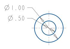
UNLESS OTHERWISE SPECIFIED, **ALB Materials Inc. DIMENSIONS ARE IN INCHES** TITLE: **TOLERANCES:** FRACTIONAL 0.030 **Ring/Tube Magnet** ANGULAR: 0.5 TWO PLACE DECIMAL 0.010 THREE PLACE DECIMAL 0.002 DWG. NO. SIZE **REV RX088 MATERIAL** SCALE: 1:1 DO NOT SCALED RAWING SHEET 1 OF 1
