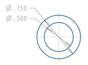
UNLESS OTHERWISE SPECIFIED, **ALB Materials Inc. DIMENSIONS ARE IN INCHES** TITLE: **TOLERANCES:** FRACTIONAL 0.030 **Ring/Tube Magnet** ANGULAR: 0.5 TWO PLACE DECIMAL 0.010 THREE PLACE DECIMAL 0.002 DWG. NO. SIZE **REV RC86 MATERIAL** SCALE: 2:1 DO NOT SCALED RAWING SHEET 1 OF 1 SEE PRODUCT PAGE
