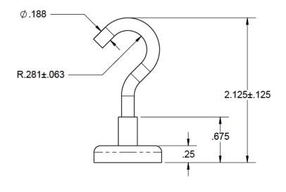
**ALB Materials Inc** UNLESS OTHERWISE SPECIFIED. DIMENSIONS ARE IN INCHES TITLE: MOUNTING MAGNET STYLE E TOLERANCES: FRACTIONAL ± 0 030 ANGULAR: ± 1° TWO PLACE DECIMAL ± 0.004 THREE PLACE DECIMAL ± 0.004 SIZE DWG. NO. **REV** MMS-E-X0 MATERIAL SEE CHART DO NOT SHEET 1 OF 1 FINISH SCALE: 1:1 SEE NOTES SCALE DRAWING
