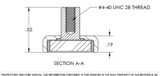
**ALB Materials Inc** UNLESS OTHERWISE SPECIFIED. DIMENSIONS ARE IN INCHES TITLE: MOUNTING MAGNET STYLE D TOLERANCES: FRACTIONAL ± 0 030 ANGULAR: ± 0.5° SIZE DWG. NO. TWO PLACE DEC MAL ± 0.010 THREE PLACE DECIMAL ± 0.005 MATERIAL SEE PRODUCT PAGE DO NOT SCALE DRAWING
