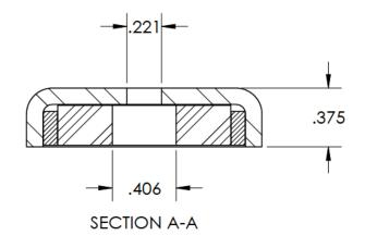
TOLERANCES: FRACTIONAL ± 0 030 ANGULAR: ± 0 5° TWO PLACE DEC MAL ± 0.010 THREE PLACE DECIMAL ± 0.005
