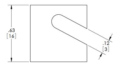
**ALB Materials Inc** D MENSIONS SHOWN AS: inches TITLE: [millimeter] MOUNTING MAGNET STYLE F TOLERANCES: FRACTIONAL ± 0 030 ANGULAR: ± 0.5° SIZE DWG. NO. REV TWO PLACE DEC MAL ± 0.010 THREE PLACE DECIMAL ± 0.005 MM-F-16 MATERIAL SEE PRODUCT PAGE DO NOT SCALE DRAWING SCALE: 3:1 SHEET 1 OF 1 FINISH SEE PRODUCT PAGE
