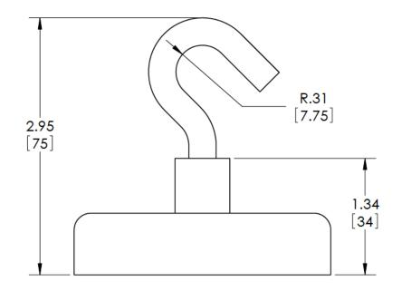
**ALB Materials Inc** DIMENSIONS SHOWN AS: inches TITLE: [millimeters] MOUNTING MAGNET STYLE E TOLERANCES: FRACTIONAL ± 0 030 ANGULAR: ± 0.5° SIZE DWG. NO. REV TWO PLACE DEC MAL ± 0.010 THREE PLACE DECIMAL ± 0.005 MM-E-75 MATERIAL SEE PRODUCT PAGE DO NOT SCALE DRAWING SCALE: 1:1 SHEET 1 OF 1 FINISH SEE PRODUCT PAGE
