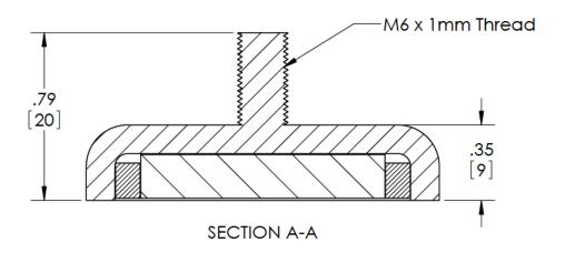
**ALB Materials Inc** DIMENSIONS SHOWN AS: inches TITLE: [millimeters] MOUNTING MAGNET STYLE C TOLERANCES: FRACTIONAL ± 0 030 ANGULAR: ± 0.5° SIZE DWG. NO. REV TWO PLACE DEC MAL ± 0.010 THREE PLACE DECIMAL ± 0.005 MM-C-42 MATERIAL SEE PRODUCT PAGE DO NOT SCALE DRAWING SCALE: 2:1 SHEET 1 OF 1 FINISH SEE PRODUCT PAGE
