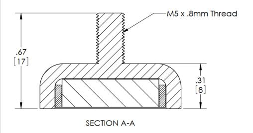
**ALB Materials Inc** DIMENSIONS SHOWN AS: inches TITLE: [millimeters] MOUNTING MAGNET STYLE C TOLERANCES: FRACTIONAL ± 0 030 ANGULAR: ± 0.5° SIZE DWG. NO. REV TWO PLACE DEC MAL ± 0.010 THREE PLACE DECIMAL ± 0.005 MM-C-25 MATERIAL SEE PRODUCT PAGE DO NOT SCALE DRAWING SHEET 1 OF 1 FINISH SCALE: 3:1 SEE PRODUCT PAGE
