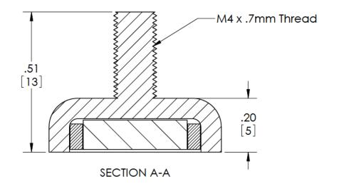
inches TITLE: [millimeters] MOUNTING MAGNET STYLE C TOLERANCES: FRACTIONAL ± 0 030 ANGULAR: ± 0.5° SIZE DWG. NO. TWO PLACE DEC MAL ± 0.010 THREE PLACE DECIMAL ± 0.005 MM-C-16 MATERIAL SEE PRODUCT PAGE DO NOT SCALE DRAWING SCALE: 4:1 SHEET 1 OF 1 FINISH SEE PRODUCT PAGE
