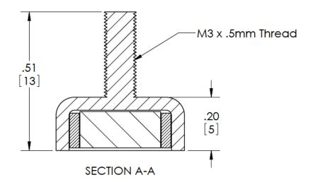
**ALB Materials Inc** DIMENSIONS SHOWN AS: inches TITLE: [millimeters] MOUNTING MAGNET STYLE C TOLERANCES: FRACTIONAL ± 0 030 ANGULAR: ± 0.5° SIZE DWG. NO. **REV** TWO PLACE DEC MAL ± 0.010 THREE PLACE DECIMAL ± 0.005 MM-C-12 MATERIAL SEE PRODUCT PAGE DO NOT SCALE DRAWING SHEET 1 OF 1 FINISH SCALE: 4:1 SEE PRODUCT PAGE
