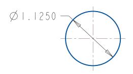
UNLESS OTHERWISE SPECIFIED, **ALB Materials Inc. DIMENSIONS ARE IN INCHES** TITLE: **TOLERANCES:** FRACTIONAL 0.030 **DISC/CYLINDER MAGNET** ANGULAR: 0.5 TWO PLACE DECIMAL 0.010 THREE PLACE DECIMAL 0.002 DWG. NO. SIZE
