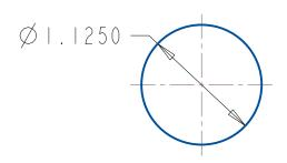
UNLESS OTHERWISE SPECIFIED, **ALB Materials Inc.** DIMENSIONS ARE IN INCHES TITLE: **TOLERANCES:** FRACTIONAL 0.030 **DISC/CYLINDER MAGNET** ANGULAR: 0.5 TWO PLACE DECIMAL 0.010 THREE PLACE DECIMAL 0.002 DWG. NO. SIZE
