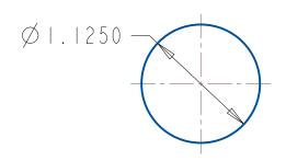
UNLESS OTHERWISE SPECIFIED, **ALB Materials Inc.** DIMENSIONS ARE IN INCHES TITLE: **TOLERANCES:** FRACTIONAL 0.030 **DISC/CYLINDER MAGNET** ANGULAR: 0.5 TWO PLACE DECIMAL 0.010 THREE PLACE DECIMAL 0.002
