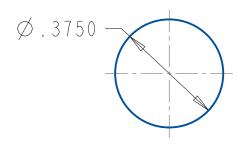
UNLESS OTHERWISE SPECIFIED, **ALB Materials Inc. DIMENSIONS ARE IN INCHES** TITLE: **TOLERANCES:** FRACTIONAL 0.030 **DISC/CYLINDER MAGNET** ANGULAR: 0.5 TWO PLACE DECIMAL 0.010 THREE PLACE DECIMAL 0.002 SIZE DWG. NO. **REV D69 MATERIAL** SCALE: 3:1 DO NOT SCALED RAWING SHEET 1 OF 1 SEE PRODUCT PAGE
