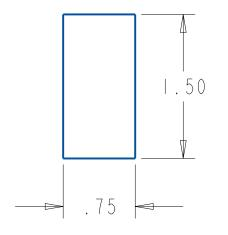
UNLESS OTHERWISE SPECIFIED, **ALB Materials Inc. DIMENSIONS ARE IN INCHES** TITLE: **TOLERANCES:** FRACTIONAL 0.030 **Block/Bar/Cube Magnet** ANGULAR: 0.5 TWO PLACE DECIMAL 0.010 THREE PLACE DECIMAL 0.002 DWG. NO. SIZE **REV BX8CC MATERIAL**
