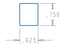
UNLESS OTHERWISE SPECIFIED, **ALB Materials Inc. DIMENSIONS ARE IN INCHES** TITLE: **TOLERANCES:** FRACTIONAL 0.030 **Block/Bar/Cube Magnet** ANGULAR: 0.5 TWO PLACE DECIMAL 0.010 THREE PLACE DECIMAL 0.002 DWG. NO. SIZE **REV BCAC MATERIAL**
