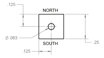
**ALB Materials Inc** UNLESS OTHERWISE SPECIFIED. DIMENSIONS ARE IN INCHES TITLE: **BLOCK MAGNET** TOLERANCES: FRACTIONAL ± 0 030 ANGULAR: ± 0.5° SIZE DWG. NO. **REV** TWO PLACE DEC MAL ± 0.010 THREE PLACE DECIMAL ± 0.005 B444-1 MATERIAL SEE PRODUCT PAGE DO NOT SHEET 1 OF 1 FINISH SCALE: 4:1 SEE PRODUCT PAGE SCALE DRAWING
